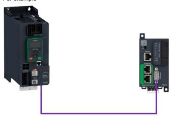
The drive is controlled from the communication (CANopen) but the reference value is adjusted with analog input 1. The control word comes from the controller and is written according to CiA 402 profile.
